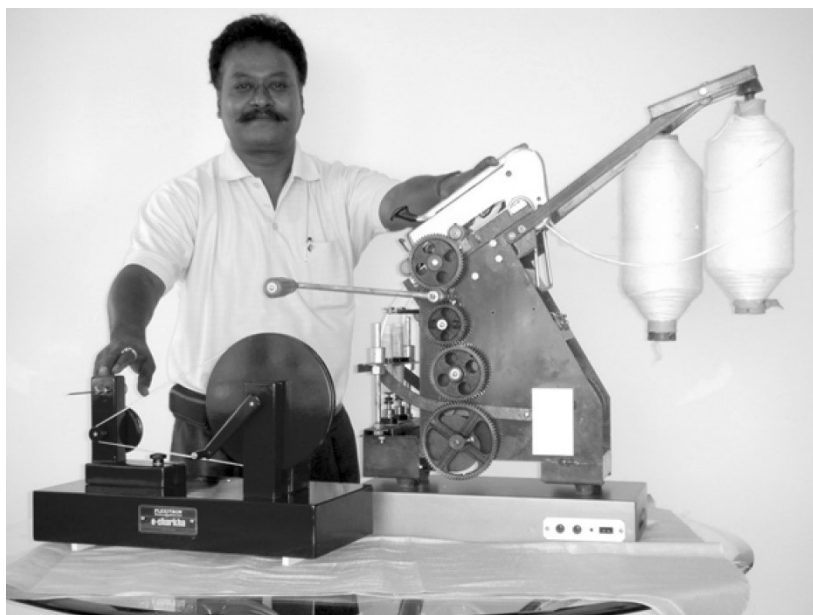
Figure 5 – Conventional and modified e-charkha
